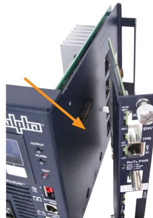
Fig. 5, Connecting the Transponder to the Inverter Module
