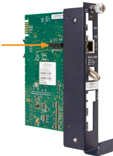
Fig. 4, The 18-pin Connector
